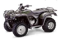
Four- or six-wheeled vehicle equipped with an engine and designed for off-road use.
